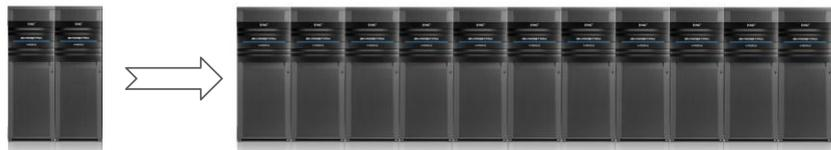
**VMAX 20K: A Scalable High-End Storage Array—VMAX 20K can be configured with 48 to 3,200 drives for a maximum capacity of up to two petabytes. The multi-engine storage system can non-disruptively scale from one to eight VMAX Engines. Systems are configured around a central system bay and adjacent storage bays of up to 240 3.5" drives each or up to 400 2.5" drives.**
