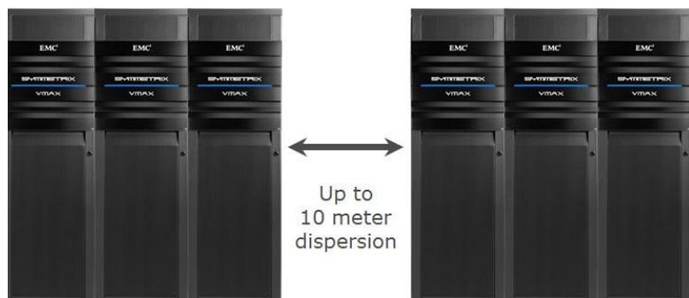
Dispersed array technology allows system bays and their associated storage bays to be separated as a unit by up to 10 meters of rack-to-rack distance allowing deployment in space constrained data centers
