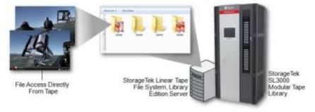
Further, StorageTek Linear Tape File System, Library Edition improves workflow efficiency. Users can drag and drop files among tape storage, flash storage, and disk storage devices without the use of specialized or expensive tape backup or archive software. Another time-saving step is that you don't have to remount tape cartridges to retrieve index data or cartridge information.
